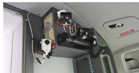
Figure 9: Cockpit LH side Video Cameras
